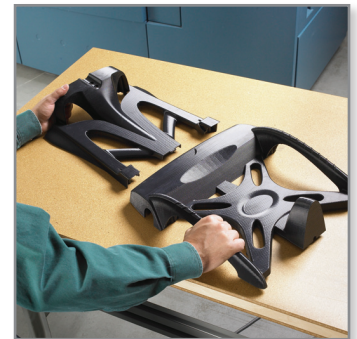
Image 2: The carrier rack prototype was built in two pieces and assembled.
